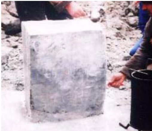
Fig. 3. Specimen preservation by waxing
