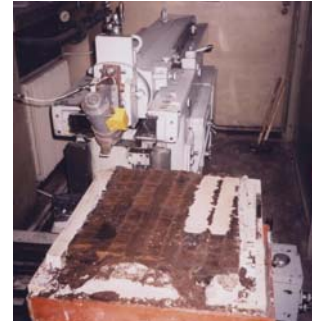
Fig. 8. Plasticine mold cutting
