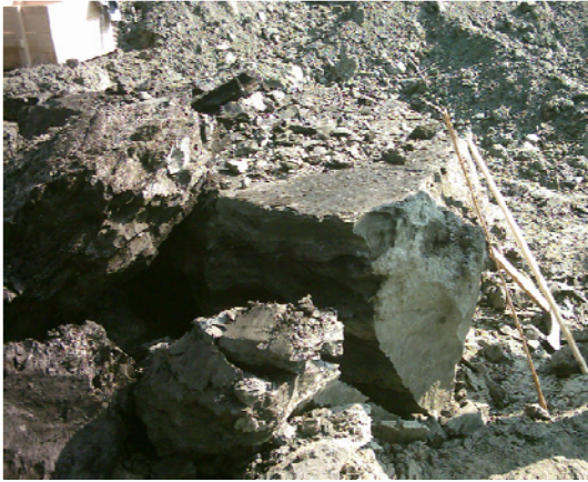
Fig. 1. Extracted block for specimen modeling
